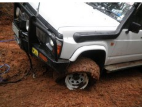
This was one of two tyres that popped a bead in the muddy conditions
